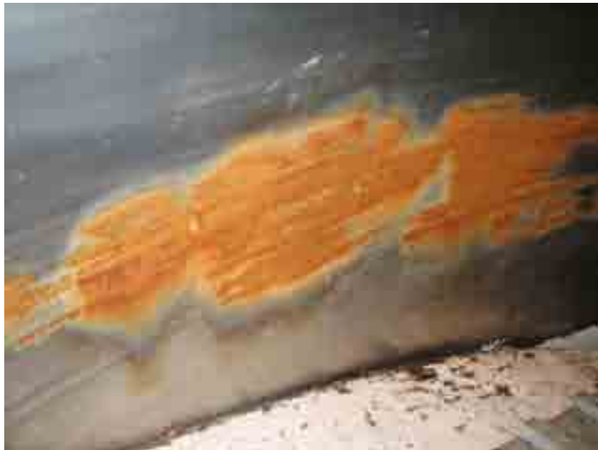
Picture of Turbine Blade Scrape with Liner Notice White-Blue Area on Stainless Steel Liner due to Heat
